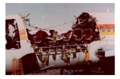
In April 28,1988, a 737-200 series became the world's first convertible when 18 ft. of front upper fuselage and, sadly, one flight attendant, departed the aircraft at 24,000 ft. altitude.
